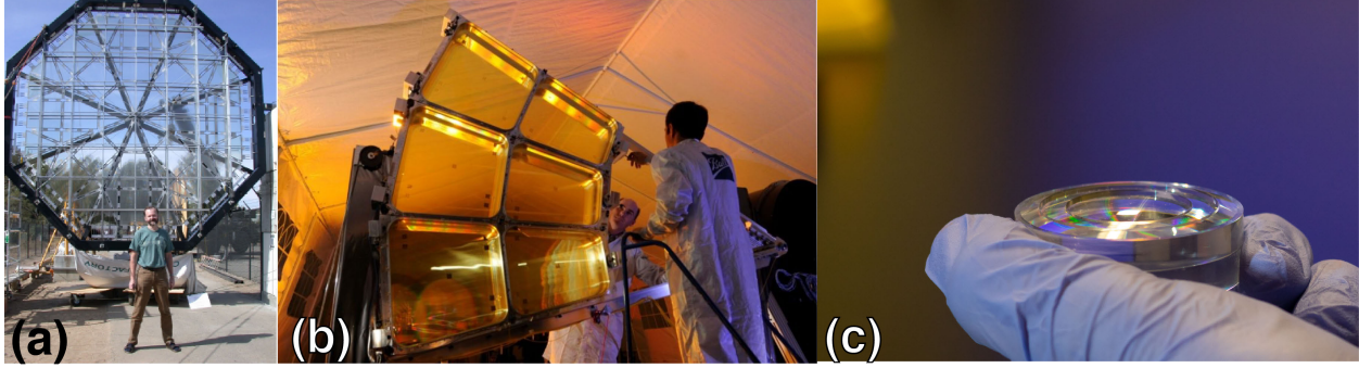
Figure 5: (a) 5m diameter Eyeglass prototype using 72 single-order diffractive optical elements [18]. (b) MOIRE test segment, using single-order diffractive optics lithographically replicated to membranes [3]. This DARPA-funded project aims to create low-cost, ultralight, 25m-diameter space telescopes. (c) MODE lens prototype developed by our team [1]. MODE lenses provide much broader wavelength coverage and enable faster optical systems than single-order diffractive lenses.
